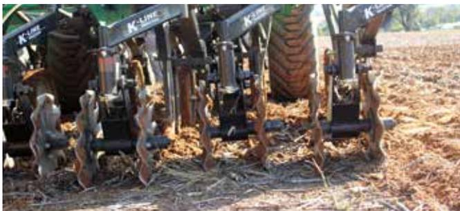
In-frame coulters are constructed of rolled hollow steel to reduce the weight on seeder frames and drawbars while maintaining the unit's strength. Coulters kits rely on adjustable springs to customise the penetration level to the type of stubble and the soil placement needs of the seeding crop.
