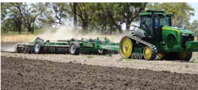
The Speedtiller® accomplishes residue incorporation by utilizing a two-part system – first chopping the residues into manageable pieces and shifting the dirt with an offset disc, and then mixing the dirt and residues together into a finished paddock surface, leaving the seedbed ready for planting. This two-step approach provides the residue incorporation farmers need to reap the benefits of better crop health and higher yields.
