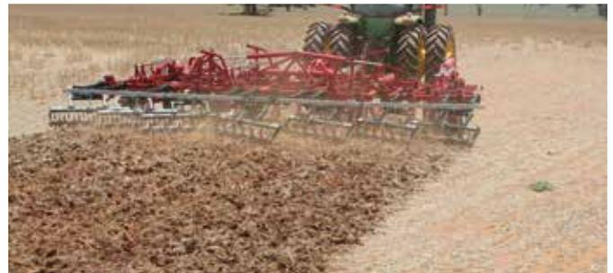
Spring tine harrows, with their scraping movement, are better suited for lighter stubble and soil, and seed types that require less soil disturbance. Standard rotary harrows, with their rotating gangs of metal tines in a diagonal configuration, penetrate more deeply into stubble and provide greater soil disturbance. These rotary harrows are especially popular as a trailing implement for ploughs, as they further disperse stubble while simultaneously levelling seedbeds for planting.
