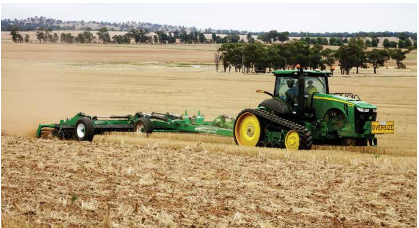
Residue issues made easy – 9.5m Speedtiller Powerflex in wheat stubble, Parkes NSW
