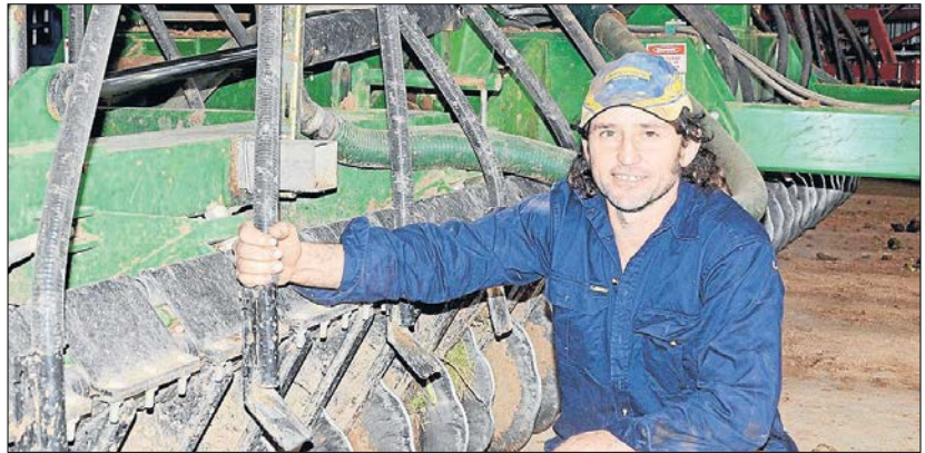
Canowindra mixed farmer Domonic Pace with his double disc machine which he has fitted with a Simplicity 2500 FM2 double bin airseeder, which allows him to sow while tilling.
