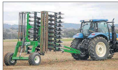
The Speedtiller has been developed to assist in cutting up and incorporating heavy residues into the top layers of soil to increase soil organic matter and improve soil performance. Increased soil organic matter is necessary for microbial activity in the soil and for nutrient efficiency.
