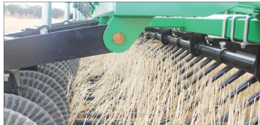
The Trashcutter's™ advanced design lays the stubble to one side before slicing and bruising it with self-sharpening discs into short lengths.
