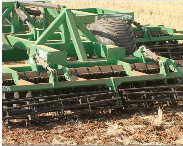
The Speedtiller® assists in cutting up and incorporating heavy residues into topsoils.
